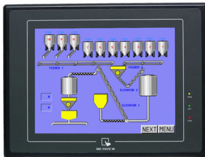
Figure 1.12 An HMI device displaying the plant mimic diagram; Picture courtesy Wienview
