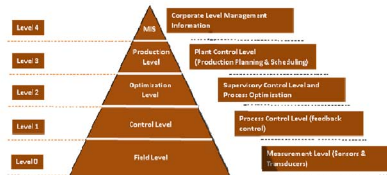
Figure 1.10 Five levels of automation hierarchy of a (hierarchical) computer based process control system
