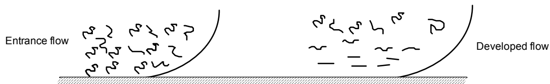
Figure 3-12: Polymers as drag reducers; low viscosity develops at the wall.
